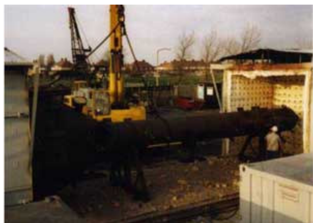
Mannings Southport base can offer an on-site 50 tonne capacity contract heat treatment furnace facility capable of temperature up to 1100 °C, together with a variety of smaller furnaces and low temperature ovens
