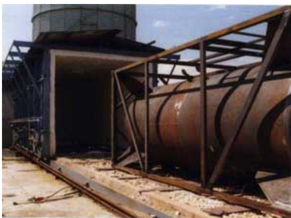
Mannings Southport base can offer an on-site 50 tonne capacity contract heat treatment furnace facility capable of temperature up to 1100 °C, together with a variety of smaller furnaces and low temperature ovens
