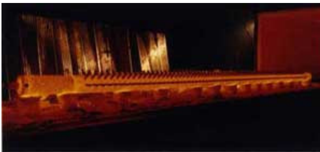
Heat treat of 13M long stainless steel header for West Burton Power Station U.K. soak temperature 1070 °C and rapid air cool
