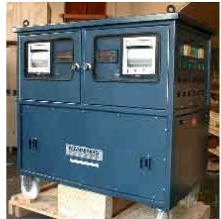
150kVA NON STANDARD HEAT TREATMENT CENTRE
